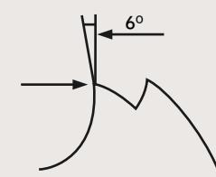
Designed for cutting steel bar. It has unique tooth angle and strength with powerful cutting performance in cutting reinforcing steel bars.
