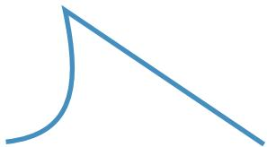
Regular tooth blades are most commonly used for all general purpose metal sawing. The face of the tooth is straight ( $0^\circ$ ,  $7^\circ$  &  $10^\circ$  rake angle).
