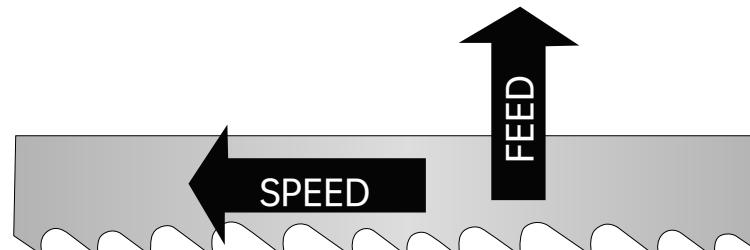
Burned heavy chips- reduce feed/speed.
